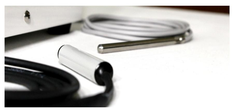
The probes, one for temperature and one for humidity, can be placed in the Grow Box in specific points, to have a more effective reading of the growth environment and improve where necessary.
